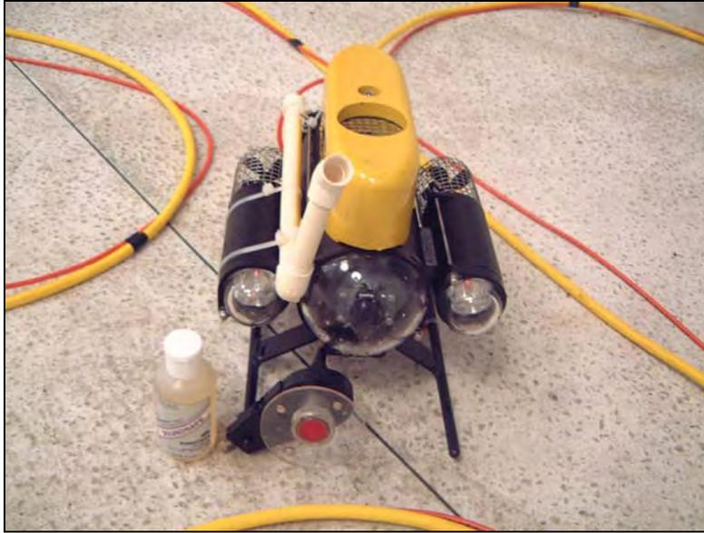
**Figure 9.17. VideoRay ROV rigged for interior oil collection (NPS Photo by Brett Seymour).**
