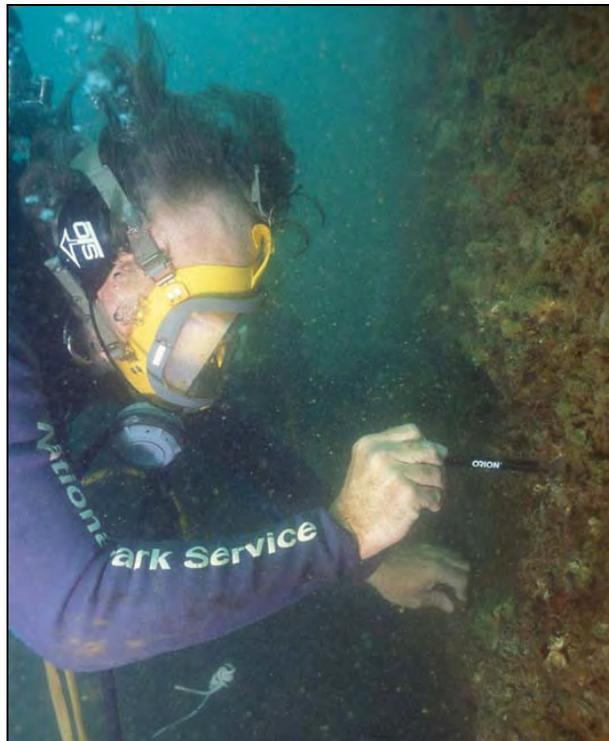
Figure 5.18. Measuring  $E_{\text{corr}}$  and pH through *Arizona*'s concretion (NPS Photo by Brett Seymour).
