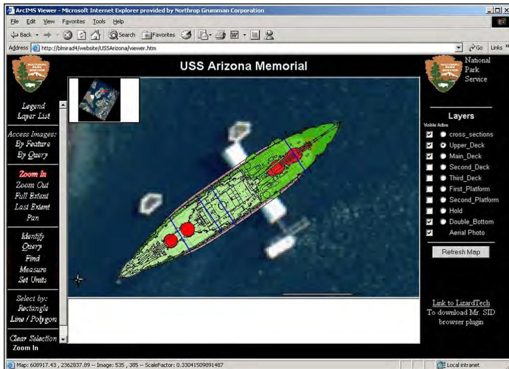
Figure 9.40. Georectified blueprints of USS *Arizona* (Image from USAR GIS Project).
