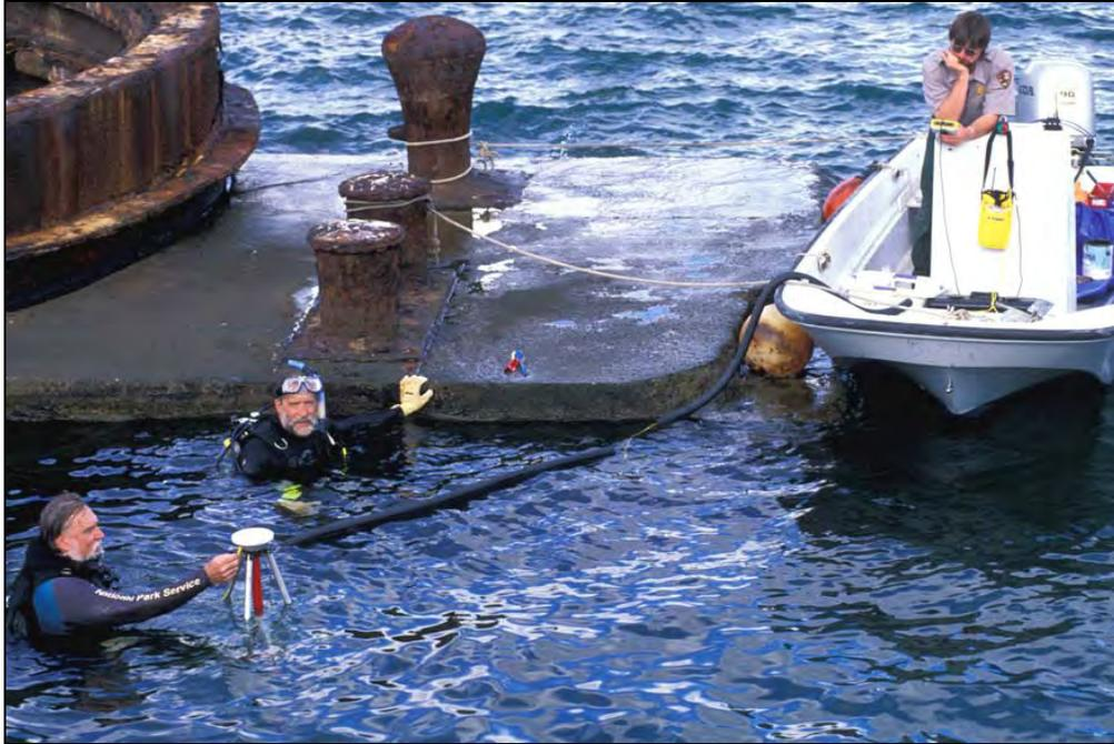
**Figure 9.9.** GPS surveying “Superpoint #2,” forward of barbette no. 3 (NPS Photo by Brett Seymour).
